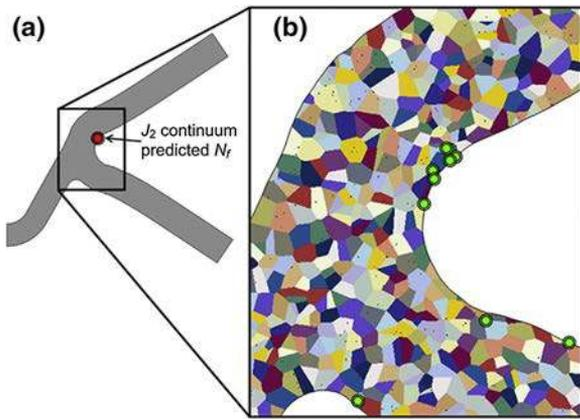
**FIGURE 8.** Fatigue-life assessment of a cobalt chromium Medinol NIR™ stent. (a) Predicted site of fatigue failure for the  $J_2$  continuum sub-model and (b) predicted sites of fatigue crack initiation for the crystal plasticity sub-model. Reprinted from Ref. 82, with permission from Elsevier.
