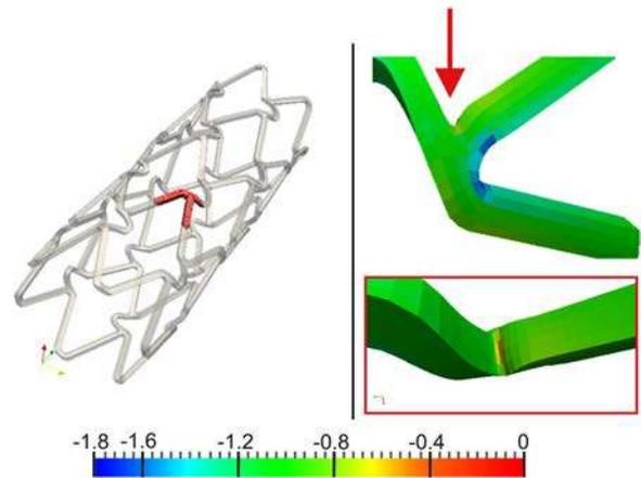
**FIGURE 7.** Fatigue-life assessment of a 316L stainless steel Medinol NIR™ stent. Application of the Dang Van criterion to the stent strut (at the top). Isovalues of the Dang Van parameter (negative values indicate no failure; positive values indicate failure). Zoom of the region (at the bottom) where the critical points are located. Reprinted from Ref. 5, with permission from Elsevier.
