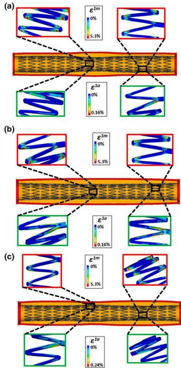
**FIGURE 9.** Fatigue-life assessment of a Nitinol peripheral stent. Contour plots of mean and alternating first principal strain for each plaque shape in case of cyclic axial compression: (a) plaque with high sharpness; (b) plaque with low sharpness, and (c) plaque with a double peak. Values of mean and alternating strain are reported in the red and green boxes, respectively. Reprinted from Ref. 24, with permission from Elsevier.
