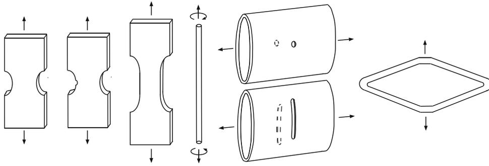
**FIGURE 6.** Geometries of the microscopic components usually tested in the literature and corresponding loading conditions; see, e.g., Refs. 66,74,82,88.
