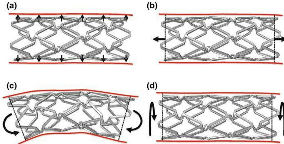
**FIGURE 4. Schematic examples of cyclic loading conditions adopted in the mechanical analysis of stents. (a) Diastole–systole; (b) compression; (c) bending; and (d) torsion.**
