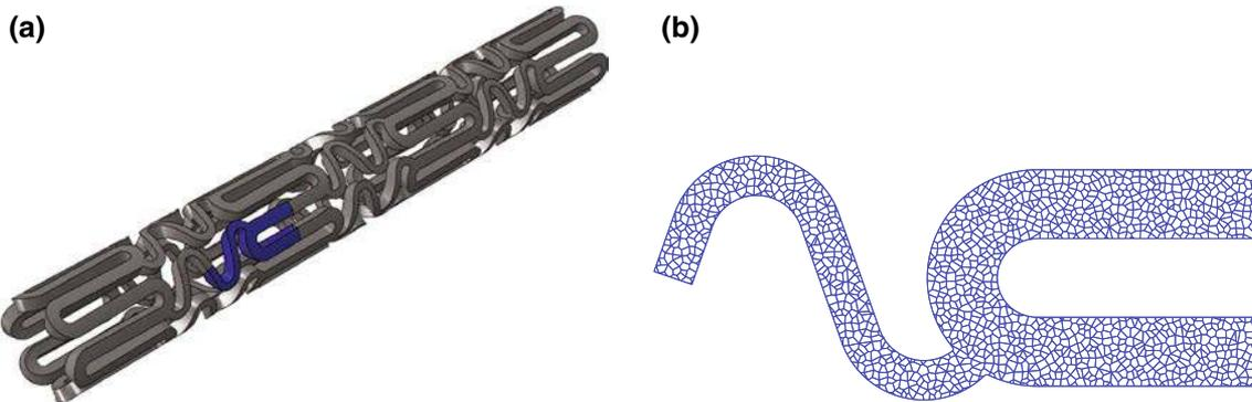
**FIGURE 5. (a) Cypher stent geometry used in the three-dimensional homogeneous model (the blue domain highlights one of the unit cells). (b) Example of a unit cell geometry used in the two-dimensional micromechanical model, containing approximately 1500 grains (personal communication of Dr. Raphael Guerchais).**
