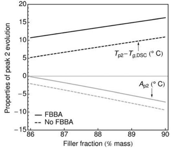
**Figure 9.** Influence of filler fraction on  $T_{p2}(2\%) - T_{p2}(0\%)$  and  $A_{p2}(2\%) - A_{p2}(0\%)$ , (NCO/OH=0.95, plasticizer=20% mass of the binder). As the material is submitted to a prestrain, ( $T_{p2}$  increases  $T_{p2}(2\%) - T_{p2}(0\%) > 0$ ) regardless of the level chosen for the DoE factors and  $A_{p2}$  decreases ( $A_{p2}(2\%) - A_{p2}(0\%) < 0$ ) for almost all of the materials.  $A_{p2}(2\%) - A_{p2}(0\%)$  decreases as the filler fraction increases.
