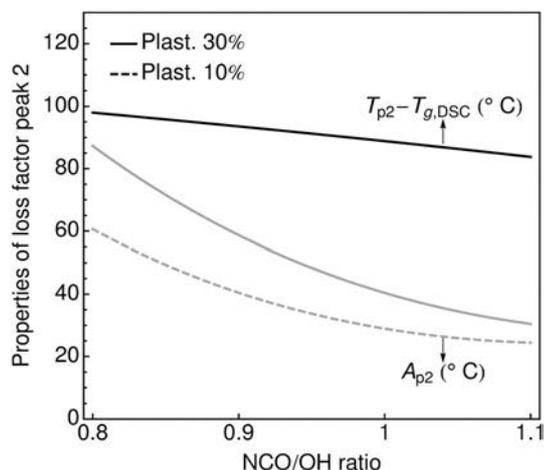
**Figure 6.** Influence of NCO/OH ratio and plasticizer content on  $T_{p2}-T_{g,DSC}$  and  $A_{p2}$  (filler fraction = 88% mass, FBBA present, plasticizer in % mass of the binder). The area  $A_{p2}$  decreases with an increase of the NCO/OH ratio and increases with the plasticizer content.  $T_{p2}-T_{g,DSC}$  decreases as the NCO/OH ratio increases. The plasticizer content has no influence on  $T_{p2}-T_{g,DSC}$ .
