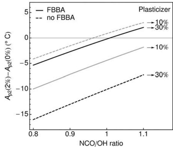
**Figure 10.** Influence of NCO/OH ratio, plasticizer content, and presence of FBBA, on  $A_{p2}(2\%) - A_{p2}(0\%)$  (filler fraction=88% mass, plasticizer in % mass of the binder).  $A_{p2}(2\%) - A_{p2}(0\%)$  increases and tends to zero as NCO/OH ratio increases.
