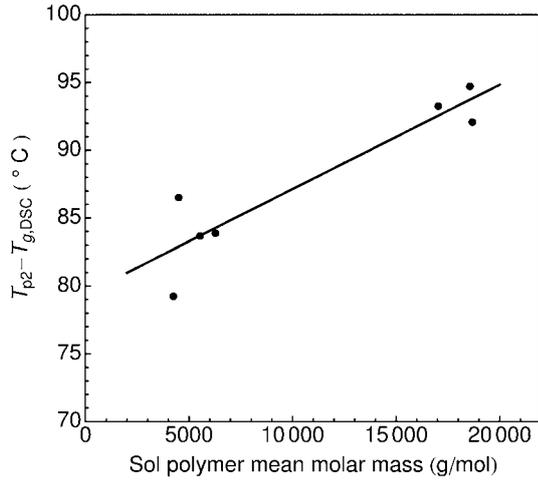
**Figure 8.** Correlation between  $T_{p2}$  and sol polymer mean molar mass for materials 0, 1, 4, 8, 11, 16, and 18. Mean molar masses determined by gel permeation chromatography [1,2].  $T_{p2}-T_{g,DSC}$  is governed by the molar mass of the sol polymer chains.
