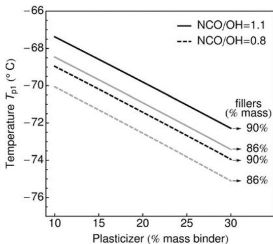
**Figure 3.** Influence of filler fraction, NCO/OH ratio, and plasticizer content on  $T_{p1}$ .  $T_{p1}$  increases with filler fraction and NCO/OH ratio, and decreases with an increase in plasticizer content.
