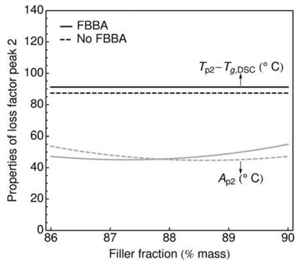
**Figure 5.** Influence of filler fraction on  $T_{p2}-T_{g,DSC}$  and  $A_{p2}$ . (NCO/OH=0.95, plasticizer=20% mass of the binder). The filler fraction has no influence on  $T_{p2}-T_{g,DSC}$ , and its effect on  $A_{p2}$  is extremely small.
