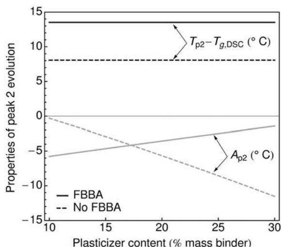
**Figure 11.** Influence of plasticizer content on  $T_{p2}(2\%) - T_{p2}(0\%)$  and  $A_{p2}(2\%) - A_{p2}(0\%)$ , (filler fraction = 88% mass, NCO/OH = 0.95). As the plasticizer content increases,  $A_{p2}(2\%) - A_{p2}(0\%)$  increases when FBBA are introduced and decreases when no FBBA are added.
