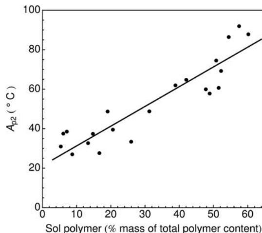
**Figure 7.** Correlation between  $A_{p2}$  and sol polymer quantity. Sol polymer fraction determined by swelling experiments [1,2]. A direct relationship between  $A_{p2}$  and the sol polymer fraction is shown for all 22 materials independently of the levels of filler fraction, NCO/OH ratio, and plasticizer content, and of the presence of FBBA.
