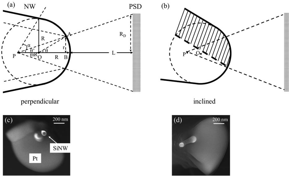
FIG. 1. Schematic illustration of projection when specimen is (a) perpendicular or (b) inclined with respect to the position sensitive detector. At a working distance  $L$  for APT with conventional configuration, the projection and analyzed volume are presented with black dot dashed line and shadow zone respectively. Top views in SEM of a specimen (NW) when the specimen tip is (c) perpendicular for STEM or (d) inclined for APT.
