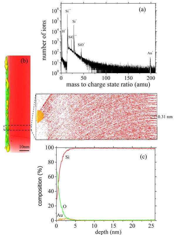
FIG. 3. (a) Mass-to-charge spectrum of Au-catalyzed VLS-grown SiNWs. (b) Atomically resolved reconstruction of an individual SiNW with a slice of atomic resolved reconstruction showing Au cluster decoration on Si facet and Si  $(111)$  planes normal to NW growth direction with inter plane distance of  $0.31 \pm 0.01$  nm. Si, Au, and O atoms are represented by red, yellow, and green, respectively. (c) Distribution of Si, Au, and O atom composition along the cross-section of individual SiNW.
