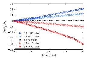
FIG. 7. Measurement of the time evolution of the normalized radius of an air bubble in water, for different values of  $\Delta P$ .
