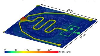
FIG. 6. Three-dimensional view of the brass mold used for the casting of the microchips. It was obtained with an optical profilometer (Zygo) by stitching images from multiple acquisitions. The height of the coating channel is 80  $\mu$ m, and its width is 300  $\mu$ m. The slope of the bubble injector is 4%.
