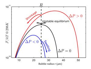
FIG. 2. Free energy of a single gas bubble of radius *R* in a weak gas-liquid solution. If  $\Delta P = 0$ , the bubble radius is stationary. The bubble shrinks if  $\Delta P > 0$  and it swells if  $\Delta P < 0$  because of gas exchange between the liquid and the bubble.
