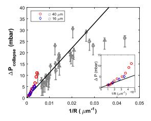
FIG. 8. Armored bubble collapse pressure as a function of the inverse radius. The black line is our model prediction, the gray symbols correspond to our experimental points, and the colored symbols correspond to measurements from Ref. [17] for two different particle diameters: 16  $\mu$ m and 40  $\mu$ m. The inset is a close-up for small values of 1/R.
