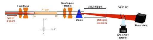
**Figure 1 | Schematic diagram of the experimental setup.** The FACET electron beam is focused by final focus quadrupoles inside a volume filled with argon gas and contained by two beryllium windows. After interacting with the plasma, electrons are transported by a quadrupole doublet towards the beam dump and deflected vertically by a dipole magnet. A Cherenkov detector is used to measure the electron energy spectrum (see the Methods for details).
