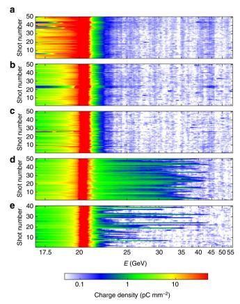
**Figure 3 | Energy gain as a function of argon pressure.** Waterfall plots of peak charge density as a function of electron energy for an argon pressure of 2 Torr (**a**), 4 Torr (**b**), 8 Torr (**c**), 16 Torr (**d**) and 32 Torr (**e**). Each waterfall plot shows 50 consecutive shots taken under the same experimental conditions (except for **e**, where only 40 shots are presented).
