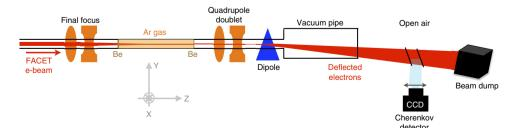
**Figure 1** | Schematic diagram of the experimental setup. The FACET electron beam is focused by final focus quadrupoles inside a volume filled with argon gas and contained by two beryllium windows. After interacting with the plasma, electrons are transported by a quadrupole doublet towards the beam dump and deflected vertically by a dipole magnet. A Cherenkov detector is used to measure the electron energy spectrum (see the Methods for details).
