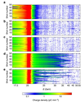
**Figure 3 | Energy gain as a function of argon pressure.** Waterfall plots of peak charge density as a function of electron energy for an argon pressure of 2 Torr (**a**), 4 Torr (**b**), 8 Torr (**c**), 16 Torr (**d**) and 32 Torr (**e**). Each waterfall plot shows 50 consecutive shots taken under the same experimental conditions (except for **e**, where only 40 shots are presented).
