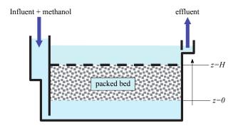
Fig. 1. Packed bed denitrifying biofilter
