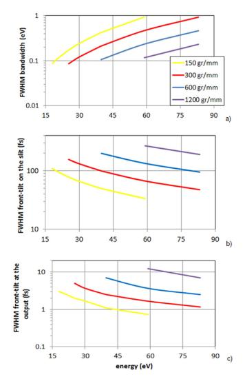
**Figure 12.** Monochromator performance with four different gratings: (a) bandwidth on 100  $\mu$ m slit; (b) front-tilt on the slit; (c) front-tilt at the output.
