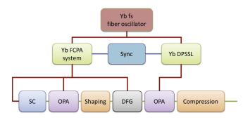
**Figure 5.** Block diagram of the MIR laser system. (DPSSL: diode pumped solid state laser, FCPA: fiber CPA, SC: supercontinuum, DFG: difference frequency generation).
