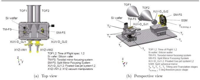
Figure 20. Graphic representation of the components arranged inside the diagnostic chamber.
