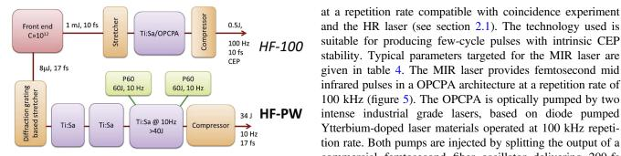
Figure 3. Block scheme of the HF laser system.
