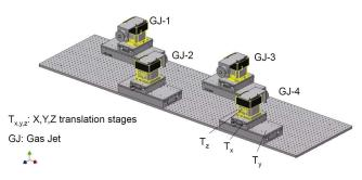
**Figure 16.** x,y,z translation stage setup on which four gas jets (GJ-1,2,3,4) can be fixed and remotely positioned with respect to the laser focus.
