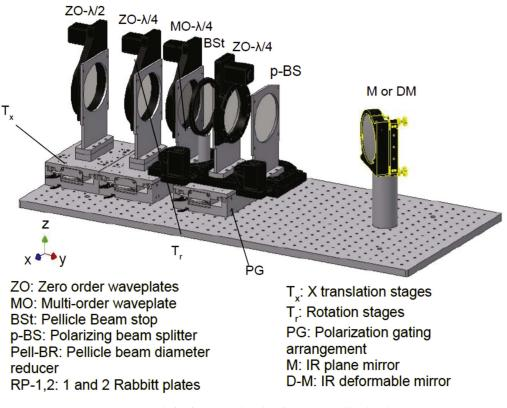
Figure 18. Polarization control and gating setup (PG2 chamber).
