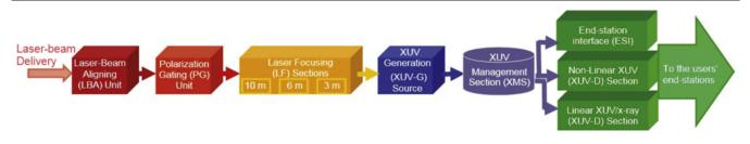
**Figure 13.** Block diagram of the SYLOS-driven users HHG beamline. The beamline consists of LBA, collinear waveplate PG, LF supporting three different focal lengths, XUV-G based on a gaseous non-linear medium, XUV-BS, steering and spectral-range-selecting section (XMS), XUV-D with subsections for XUV-CC and XUV-AC measurements, as well as a number of other diagnostics, and the end station interfacing (ESI) branch.
