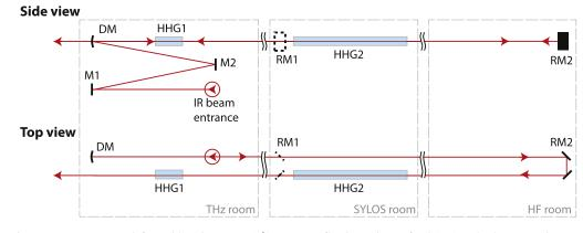
**Figure 22.** Focusing geometry. DM—deformable mirror, RM1/2—retro-reflecting mirrors for SAP1 and other operation modes, HHG1/2—HHG cell position for SAP1 and other operation modes.
