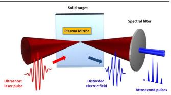
**Figure 24.** The mechanism of surface high-order harmonics generation from high intensity laser driven plasma mirror.
