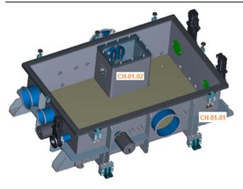
**Figure 10.** 3D layout of the main chamber of section 1. CH-01.01 hosts the optical elements and motorized movements to split and handle the two IR beams. The gas cell for the generation of attosecond pulses is hosted in CH-01.02, and is independently pumped to increase the differential pumping capabilities. The IR focusing mirror is mounted on an external chamber.
