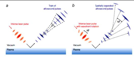
**Figure 28.** The basic principle of the attosecond lighthouse. (a) Attosecond pulse train from pulses without wavefront rotation. (b) Attosecond pulse train from pulses with wavefront rotation. [94] (2017) Figure reprinted with permission of Springer.
