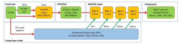
Figure 2. Block diagram for SYLOS 1 laser system.
