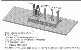
Figure 19. The optical layout of the XUV-BM chambers.
