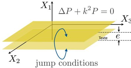
Fig. 14.3. In the homogenized problem, the Helmholtz equation applies in the whole-considered-space except in the region  $-e/2 < X_1 < e/2$  which is disregarded; the jump conditions (14.27) apply between  $X_1 = -e/2$  and  $e/2$ .
