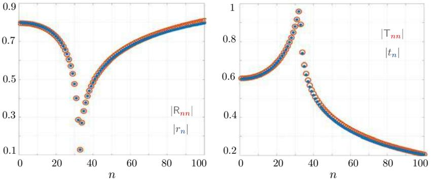
Fig. 14.12. Comparison of the reflection and transmission coefficients of the modes,  $(R_{nn}, T_{nn})$  for  $n = 1, \dots, 100$  from direct numerics (computed with a truncation  $N = 3000$ ), and  $(r_n, t_n)$  given by the interface model, Eqs. (14.40).
