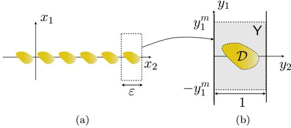
Fig. 14.2. (a) Geometry of the structured film in non dimensional coordinates  $\mathbf{x} = (x_1, x_2, x_3)$ ; (b) inner problem in coordinates  $\mathbf{y} = (y_1, y_2, y_3)$ .  $\mathcal{D}$  is the region occupied by the rigid inclusion. We define  $\mathcal{Y} = (-y_1^m, y_1^m) \times (0, 1)^2$ ,  $\mathcal{Y}_\infty = \lim_{y_1^m \rightarrow +\infty} \mathcal{Y}$ , and  $\mathbf{x}' = (x_2, x_3)$ ,  $\mathbf{y}' = (y_2, y_3)$ .
