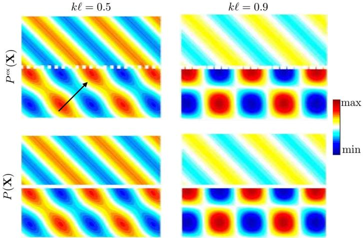
Fig. 14.6. Wavefields in the  $(X_1, X_2)$  plane for  $ke = 0.5$ ,  $kh = 1$ , and  $kl = 0.5$  or  $0.9$  (a)  $P^{\text{ex}}(\mathbf{X})$  and (b)  $P(\mathbf{X})$  coming from the interface model, Eqs. (14.32)–(14.33). The white arrow indicates the wavenumber of the incident plane wave.
