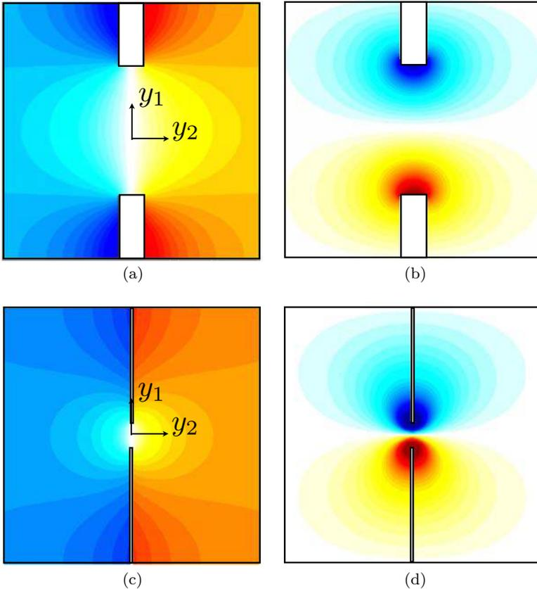
Fig. 14.14. Static fields computed for the elementary problems  $i = 1$  and 2. (a) (c)  $q^{(1)}(\mathbf{y})$  and (b) (d)  $q^{(2)}(\mathbf{y})$ . (a–b) for  $e/h = 0.1$  and  $l/h = 0.5$ , (c–d) for  $e/h = 0.01$  and  $l/h = 0.9$ .
