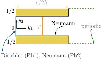
Fig. 14.13. Mode matching configuration. The solutions  $Q^-$  and  $Q^+$  are written for  $0 \leq y_1 \leq e/2h$  and  $y_1 \geq e/2h$  respectively (with proper conditions at  $y_1 = 0$ ), and the resolution involves only matching conditions at  $y_1 = e/2h$ .
