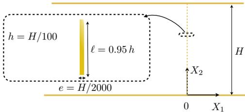
Fig. 14.9. Configuration of the rigid waveguide obstructed by a perforated screen at  $-e/2 < X_1 < e/2$ . The screen has a periodic spacing  $h = H/100$  and thickness  $e = H/2000$ . The height of the rigid material in the screen is  $l/h = 0.95$ . The guide is studied in the high frequency regime, with  $kH = 100$ .
