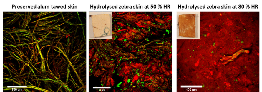
Figure 4. Nonlinear optical microscopy images of preserved alum-tawed skin, and hydrolyzed zebra skins kept at 50% RH and 80% RH, together with photographs of the zebra samples
