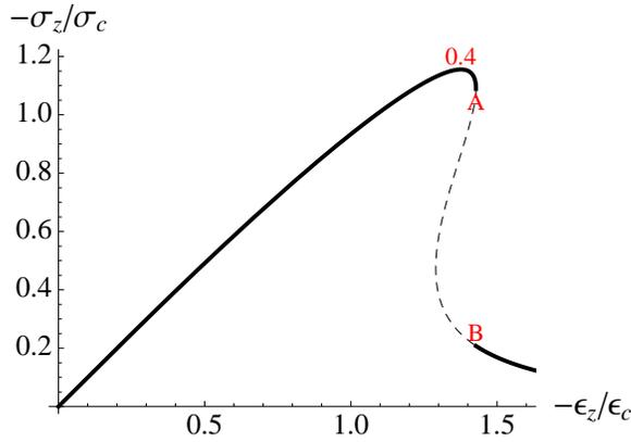
Figure 3: When  $R_1/E_0$  is large enough, the graph of  $\sigma_z$  vs  $\varepsilon_z$  contains a snap-back (here  $R_1 = 0.4E_0$ ). Consequently, when the axial strain reaches the value corresponding to the limit point **A**, the response jumps from **A** to **B**.
