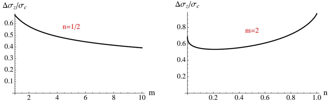
Figure 6: Dependence of the overstress  $\Delta\sigma_z$  on the exponents  $m$  and  $n$  of the model. Left, dependence on  $m$  when  $n = 1/2$ ; right, dependence on  $n$  when  $m = 2$ . In all cases  $R_1 = 0.1E_0$  and  $k = 0.2$ .
