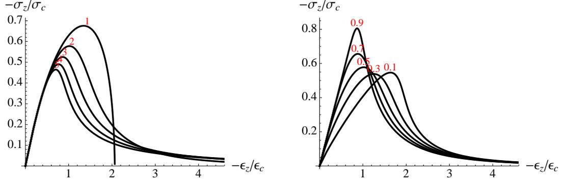
Figure 5: Influence of the exponent  $m$  (left) and  $n$  (right) on the graph of the axial stress vs the axial strain in a uniaxial compression test ( $p_0 = 0$ ). The values of  $m$  and  $n$  are indicated in red on the graph. In the left figure where  $m$  varies, one takes  $n = 1/2$ , whereas on the right figure where  $n$  varies, one takes  $m = 2$ . In all cases  $R_1 = 0.1E_0$ .
