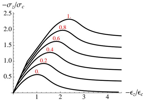
Figure 4: Graph of the axial stress vs the axial strain for different values (in red on the graphs) of the confining pressure (in fact of the ratio  $p_0/\sigma_c$ ) when  $R_1 = 0.1E_0$ . The first part (the linear part) of the graphs correspond to the hydrostatic and elastic stages.
