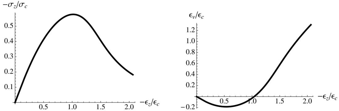
Figure 1: Graphs of the axial stress  $\sigma_z$  (left) and of the volumetric strain  $\varepsilon_v$  (right) versus the axial strain  $\varepsilon_z$  when  $R_1 = 0.1E_0$  and  $p_0 = 0$  (uniaxial compression test).
