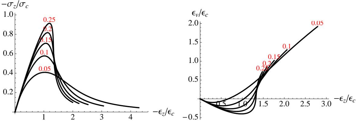
Figure 2: Influence of  $R_1/E_0$  on the graphs of the axial stress and the volumetric strain versus the axial strain when there is no confining pressure (uniaxial compression test). The value of  $R_1/E_0$  associated with each graph is indicated in red on the graph.
