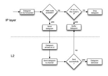
Figure 1. Link buffering process for L3 and L2
