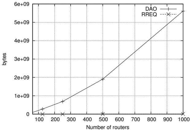
Figure 6: Extrapolated control traffic overhead for 24 hours
