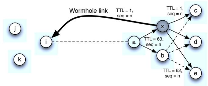
Figure 4. Pre-play attack based on TTL values.  $X$  is the malicious router which forwards the packets with reduced TTL values.
