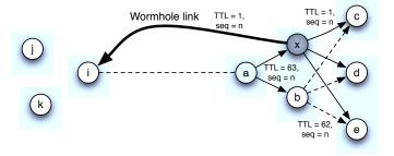
Figure 4. Pre-play attack based on TTL values. *X* is the malicious router which forwards the packets with reduced TTL values.
