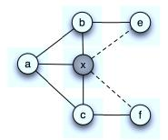
Figure 13. Multicast disruption by link spoofing: X spoofs the link to e and f.
