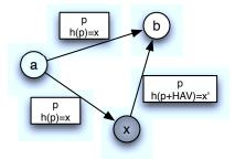
Figure 8. Attack by adding a HAV header option: The malicious router X disables duplicate packet detection by adding a HAV header option.
