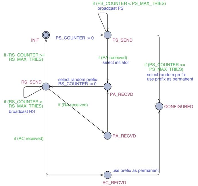
Figure 3. State machine of a *configuring* router
