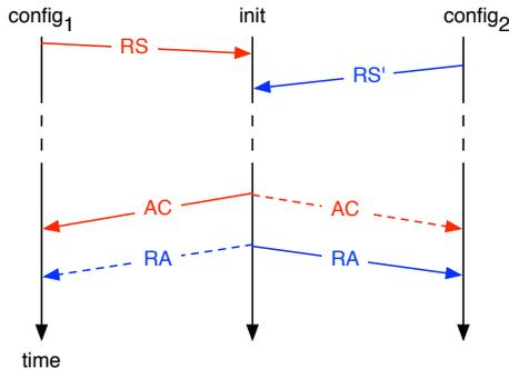
Figure 5. Two routers *config<sub>1</sub>* and *config<sub>2</sub>* having the same UUID lead to ambiguous destinations of ACs
