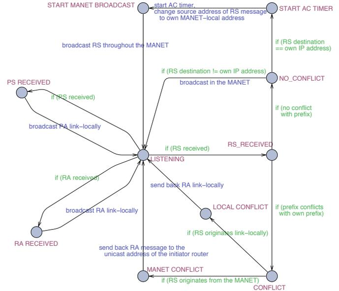
Figure 4. State machine of a *defensive* router
