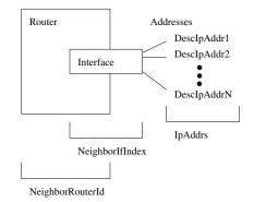
Fig. 2. The linkage between the OLSRv2 and the NHDP MIBs
