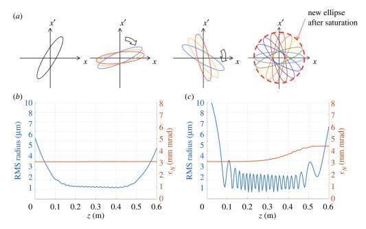
**Figure 3.** (a) Trace-space ellipse evolution for different energies (colours), red dashed circle illustrates geometrical emittance saturation. (b) and (c) RMS radius (in blue) and mean normalized emittance ( $\sqrt{\epsilon_{Nx} \cdot \epsilon_{Ny}}$ , in orange) for matched (b) and mismatched (c) cases.
