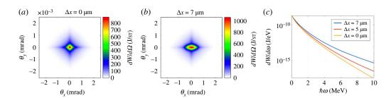
**Figure 5.** (a) Angular distribution (J/sr) of the betatron radiation emitted by both beams when no offset in the trailing was induced. (b) Angular distribution (J/sr) of the betatron radiation emitted by both beams when a 7  $\mu$  m offset is introduced along the x-axis for the trailing bunch. (c) Energy spectrum of the betatron radiation emitted by both bunches for three different offset values. (Online version in colour.)
