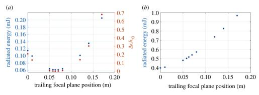
**Figure 4.** (a) Total radiated energy (blue) and relative emittance growth (orange) from the trailing bunch as a function of the focal plane position of the trailing bunch. (b) Total radiated energy from the trailing and drive bunches.
