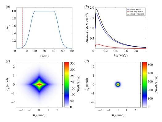
**Figure 1.** (a) Plasma density profile used for QuickPIC simulations ( $n_0 = 4 \times 10^{16} \text{ cm}^{-3}$ ). Red-dashed line shows the position of the focal plane of the trailing bunch for the matched conditions. (b) Photon energy spectrum of the radiation emitted by the trailing bunch (red), drive bunch (blue) and both (black). (c) Radiation angular distribution of the drive bunch (J/sr). (d) Radiation angular distribution of the trailing bunch (J/sr).
