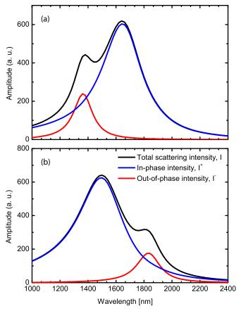
FIG. 8. Comparison of the in-phase and out-phase calculated intensities ( $I^+$  and  $I^-$ , respectively) with respect to the overall simulated scattering intensity (I) for simulations A (a) and B (b).
