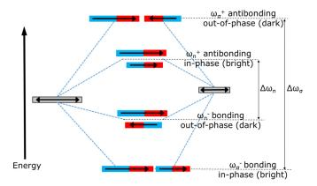
FIG. 4. Energy splitting in hybrid modes for a dipole dimer perpendicular ( $\pi$ -type stacking) and parallel ( $\sigma$ -type stacking) to the dimer axis. Red and blue colors, respectively, indicate positive and negative charge distribution.
