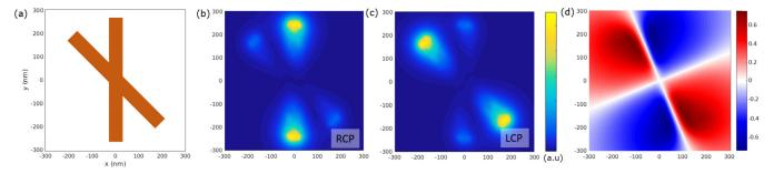
FIG. 2. Simulated response of two equal gold nanoantennas forming a cross by 45°. (a) shows the geometry and dimensions of the cross structure, which has a thickness of 50 nm. (b) and (c) show the scattered field  $|E|^2$  in a plane at 10 nm above the cross when the structure is illuminated with a plane wave of 1640 nm with right-and left-circular polarizations, respectively. In (d) we calculate the ratio  $(I_{LCP} - I_{RCP})/(I_{LCP} + I_{RCP})$ .
