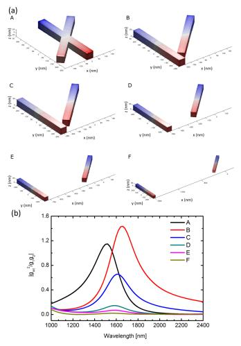
FIG. 6. (a) Different geometries of nanoantenna dimers considered in the BEM simulations. The only difference between the considered cases is the distance between the center of the nanoantennas (d), which is respectively set at 0 nm, 225 nm, 250 nm, 500 nm, 750 nm, and 1500 nm in A, B, C, D, E, and F. (b) Spectroscopic values of  $|g_{\text{int}}^2/g_1g_2|$  for the six different configurations.
