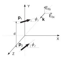
FIG. 1. Scheme of the geometry. Dimer axis and dipole vectors are perpendicular to the direction of propagation of incident light.
