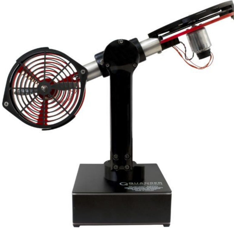
Fig. 1. The Quanser AERO half-quadrotor
