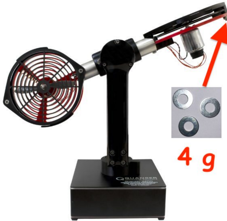
Fig. 2. Additive masses on the AERO
