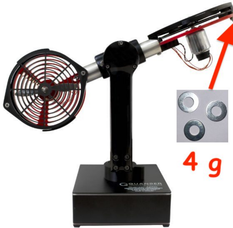
Fig. 2. Additive masses on the AERO
