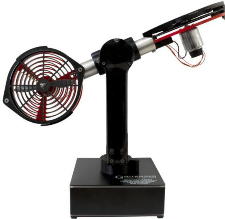
Fig. 1. The Quanser AERO half-quadrotor
