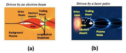
Fig.2 Nonlinear plasma wakes produced by a) an electron beam and b) a laser pulse. In both cases the drive pulses are travelling from the right to the left. In a) the black curve shows the onaxis longitudinal electric field of the wake.
