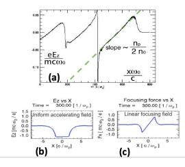
Fig.3: (a) The on axis longitudinal electric field  $E_z$ of a wake in the "bubble" regime. The slope of the accelerating field in the first bubble is  $n_r/2n_0 = \varepsilon/2$ . (b) The transverse variation of the longitudinal  $E_z$  field and (c) transverse variation of the focusing field  $F_x = (E_x - B_y)$ . In the bubble regime the  $E_z$  field is constant whereas the the focusing field is linear in the transverse direction x.
