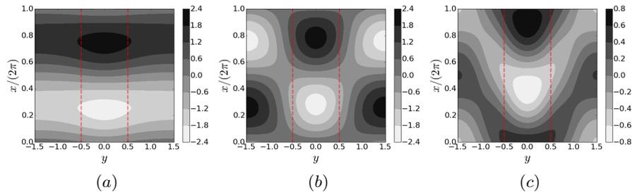
FIG. 8: Free surface deformations of unstable modes for  $Fr = 2$ ,  $l = 1$  corresponding to colored symbols on Figure 7. (a) Regime  $R_0$ ,  $U^* = 1.85$ , (b) Regime  $R_2$ ,  $U^* = 3.2$  and (c) Regime  $SF$ ,  $U^* = 6.0$ . The flag is located between the two red lines. Flag displacement amplitude is set to unity, and maximum flag displacement corresponds to  $x = 0$ .
