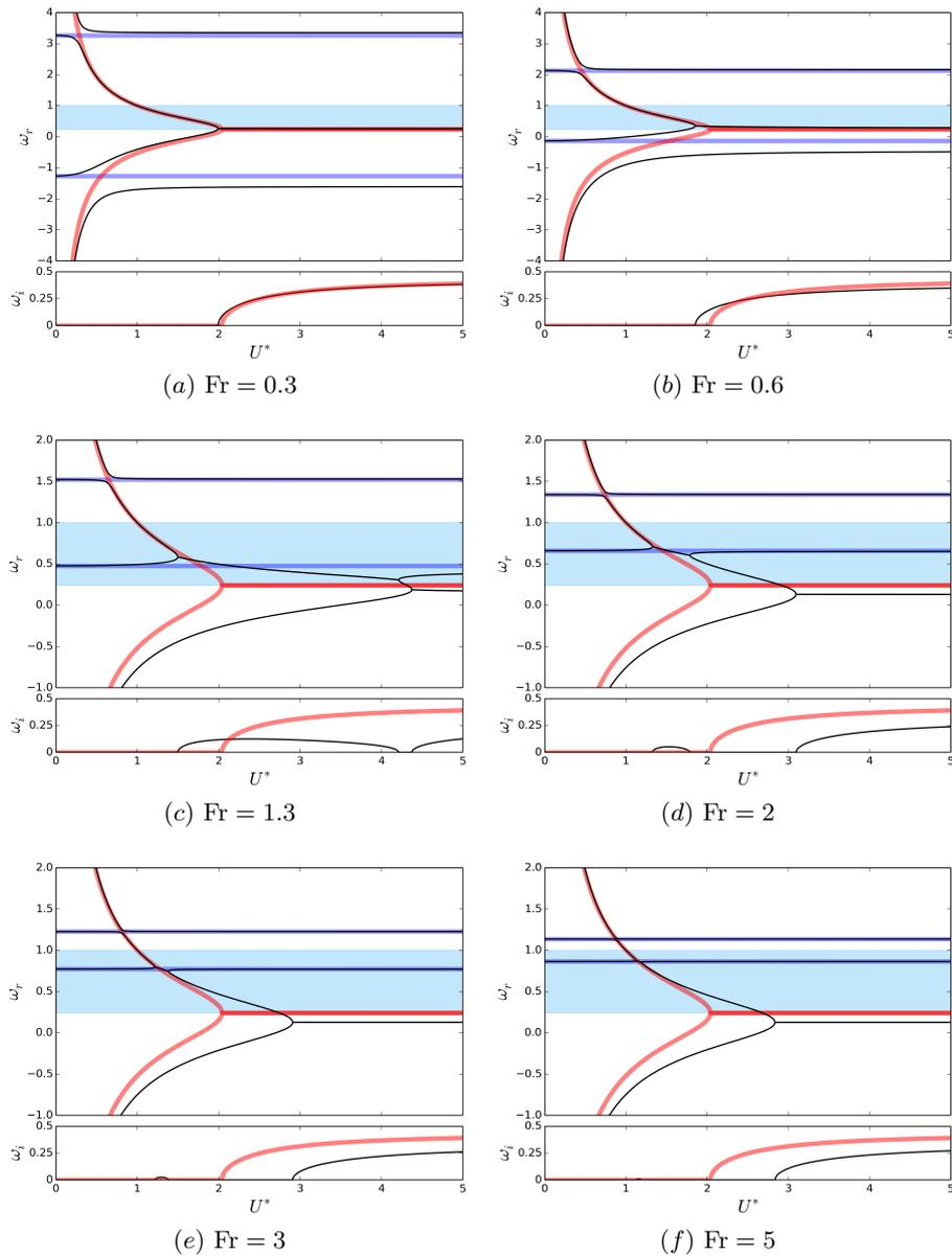
FIG. 4: Evolution with  $U^*$  of the frequencies of the fully-coupled waves (black, Eq. (20)) for various Froude numbers for  $h^* = 0.5$ . The uncoupled flag waves (red, Eq. (21)) and uncoupled gravity waves (blue, Eq. (22)) are also plotted for comparison. The shaded blue area correspond to the frequency range given by Eq. (27).
