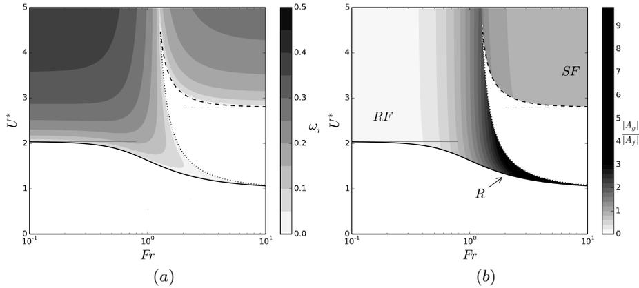
FIG. 5: Evolution of the growth rate of the unstable coupled mode (a) and corresponding amplitude ratio (b) with Fr and  $U^*$  for  $h^* = 0.5$ . Black lines correspond to velocity thresholds  $U_{c1}^*$  (plain),  $U_{c2}^*$  (dotted) and  $U_{c3}^*$  (dashed). Thin horizontal lines indicate flutter thresholds in the small-Fr (plain,  $U_c^* = 2.04$ ) and large-Fr (dashed,  $U_c^* = 2.80$ ) limits.
