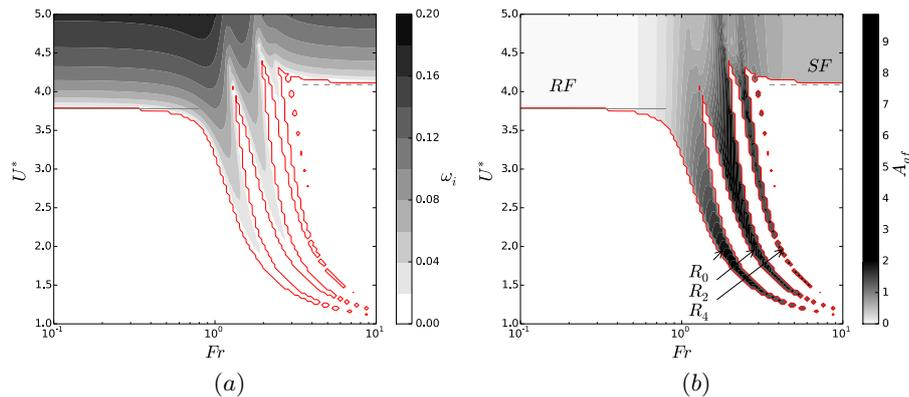
FIG. 9: Stability maps in the finite span case for  $l = 1$ . (a) Growth rate. (b) Amplitude ratio  $A_{gf} = \max[Re(A_g(y)e^{ix}/A_f)]$  as a function of the Froude number  $Fr$  and the reduced velocity  $U^*$ . The stability thresholds are indicated by red lines. Thin horizontal lines indicate flutter thresholds obtained numerically for  $Fr = 0$  (plain,  $U_c^* = 3.78$ ) and  $Fr = 10^3$  (dashed,  $U_c^* = 4.09$ ).
