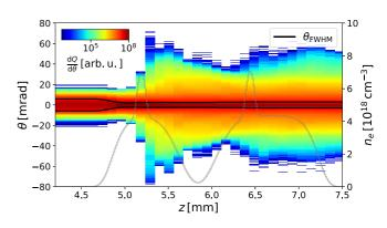
FIG. 6. Divergence evolution of the bunch while propagating through the PWFA stage. In black, the FWHM of the divergence is marked. When the bunch enters the PWFA stage and is being focused, the FWHM divergence  $\theta_{\text{FWHM}}$  reduces.
