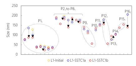
Figure 4: Evolution of precipitates and their associated zones/inclusions for L1 before and after both SSTCs. Inclusions belonging to the same mixed precipitates are inside dashed ellipses. Arrows indicate a significant increase/decrease.
