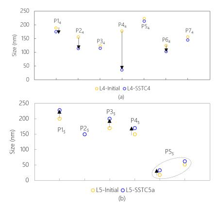
Figure 10: Precipitate size evolution for (a) L4 and (b) L5. Inclusions belonging to the same mixed precipitates are inside dashed ellipses. Arrows indicate a significant increase/decrease.
