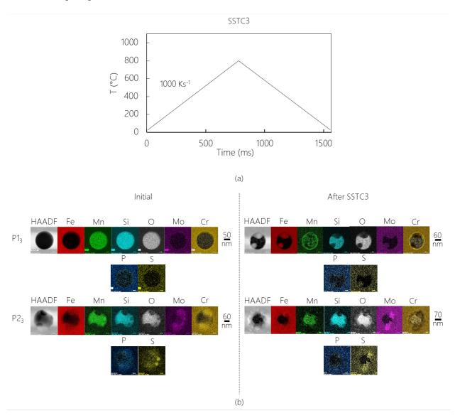
Figure 6: (a) SSTC3 single cycle up to 800°C at 1000K/s, (b) HAADF STEM images and EDS maps of the two precipitates in L3 before (same as in [30] obtained through Creative Commons Attribution 4.0 International CC by 4.0 license) and after SSTC3.
