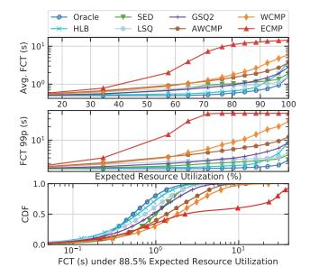
Figure 10. [Simulator] FCT comparison using 2x server capacity ratio under various traffic rates.
