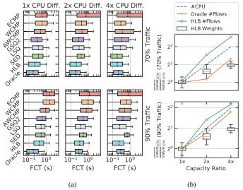
Figure 12. [Simulator] Comparison using different server capacity ratios under 70% (top) and 90% (bottom) expected resource utilisation. Figure (a) compares the FCT distribution and figure (b) compares the ratio of weights and load distribution between two groups of servers.
