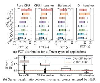
Figure 22. [Simulator] Simulation results with 3-stage application queries under 90% expected resource utilisation.
