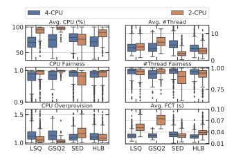
Figure 9. [Testbed] Comparison on server resource utilisations using network traces from hour 20:00 (800 queries/s) in the 24-hour Wikipedia replay.
