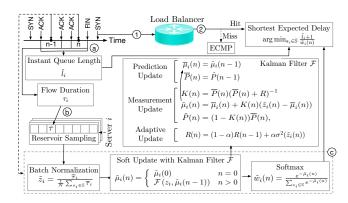
Figure 3. HLB workflow overview. Step ① and ② represent the decision making process on arrival of new flows. In step ②—ⓒ, HLB collects networking observations and periodically learns server load states.
