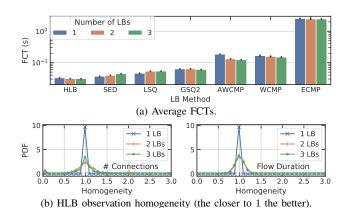
Figure 16. [Testbed] Comparison using different number of LB nodes.
