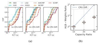
Figure 11. [Testbed] Comparison using different server capacity ratios using trace from hour 23:00 (680 queries/s). Figure (a) compares FCT CDF under 3 ratio configurations of CPU capacity differences using different LB algorithms. Figure (b) compares the server weights ratio between the two server groups generated by HLB with the actual provisioned server capacity ratios
