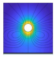
FIG. 5. Bistability of the base state: the concentration distribution and streamlines are shown for the two different branches of solutions coexisting for d = 5 and Pe = 14, showing respectively dipolar (left) and quadrupolar (right) symmetry. The relative stability of these two branches is analyzed in Sec. V C and Fig. 8; the quadrupolar branch is more unstable to longitudinal swimming modes.
