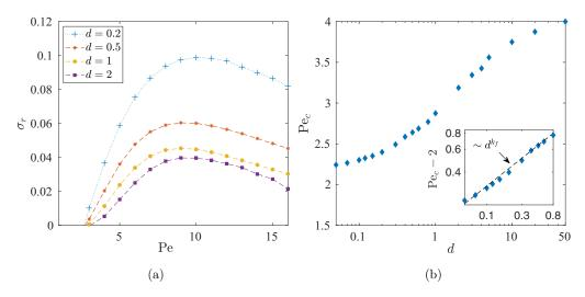
FIG. 9. (a) Evolution with Pe of the growth rate,  $\sigma_r$ , of the unstable horizontal swimming mode for small-to-moderate wall distance, d. (b) Evolution with d of the critical Péclet number for the onset of self-propulsion, Pe<sub>c</sub>. The log-log inset shows the asymptotic dependence of Pe<sub>c</sub> in the lubrication limit  $d \to 0$ , where the dashed line is a power-law fit,  $\sim d^{k_f}$ ,  $k_f \approx 0.46$ .
