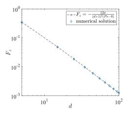
FIG. 2. The vertical force acting on the (fixed) drop as a function of its separation, d, from the wall, for Pe = 5. The symbols represent results from the numerical analysis described in Sec. III and the dashed line is the analytical approximation for the case when  $d \gg 1$  and Pe < 8.
