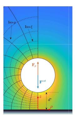
FIG. 1. An active drop levitating above a rigid wall. The equilibrium distance,  $d^*$ , is dictated by a balance between the external force,  $\mathbf{F}^{\text{ext}}$ , and the "phoretic force,"  $\mathbf{F}_p$ . The isosurfaces of constant  $\xi$  and  $\mu$  on the left half define the (body-fixed) bispherical grid. Also shown is the origin of the  $(\rho, z)$  cylindrical coordinate system.
