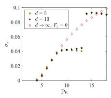
FIG. 6. Evolution of the growth rate of the unstable swimming mode for levitating droplets (forced  $F_z \neq 0$ ,  $F_x = F_y = 0$ ) for drop-wall separations d = 5 and d = 10. The results for a force-free particle in an unbounded fluid (i.e.,  $d \to \infty$ ,  $\mathbf{F} = \mathbf{0}$ ) are shown for comparison.
