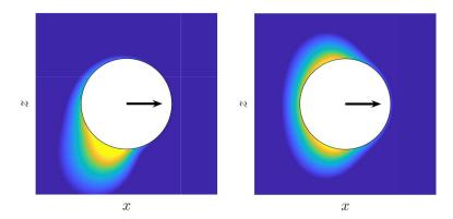
FIG. 8. Higher instability of the quadrupolar base state (right) than the dipolar base state (left), for a horizontally swimming drop (denoted by the black arrow), shown here for Pe = 14. The contours are qualitative depictions of the solute distribution around the drop in the self-propelling state, with lighter (darker) colors denoting higher (lower) concentrations.
