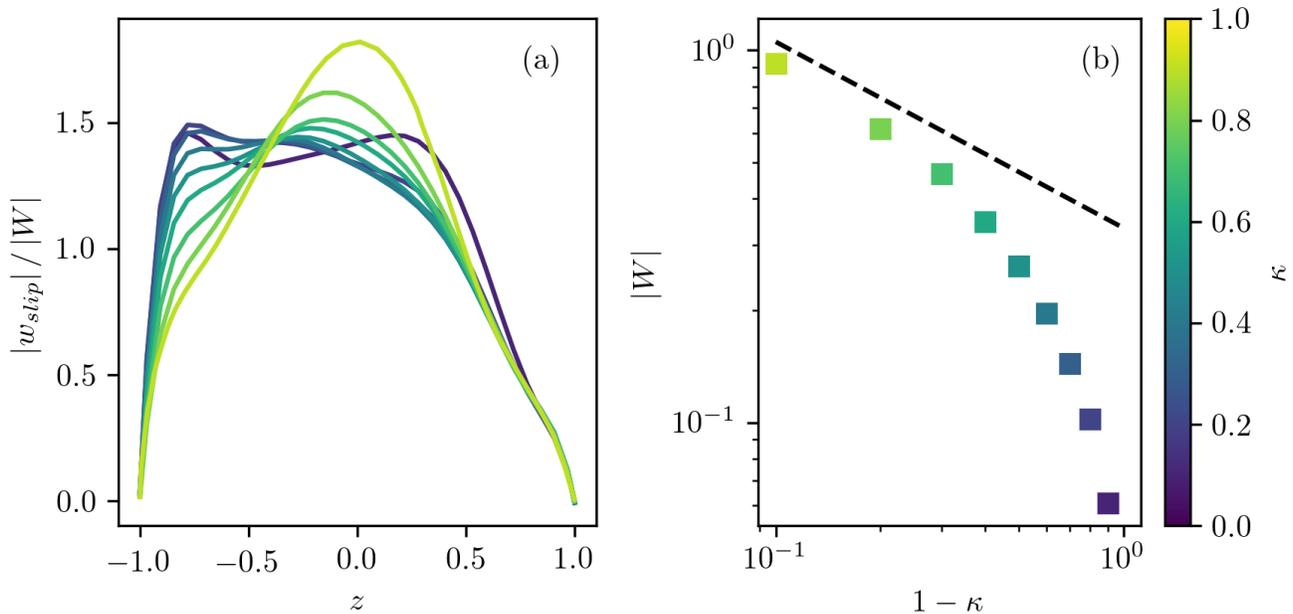
FIG. 8: (a) Distribution of the surface slip velocity normalized by the average fluid velocity in the particle-capillary gap. The results are reported for  $\kappa = n/10$  with  $2 \leq n \leq 8$ . (b) Average fluid velocity in the particle-capillary gap  $W$  at varying confinement  $\kappa$ . Results are shown here for  $Pe = 6.0$ . The dashed line corresponds to the analytical prediction, Eq. (39).
