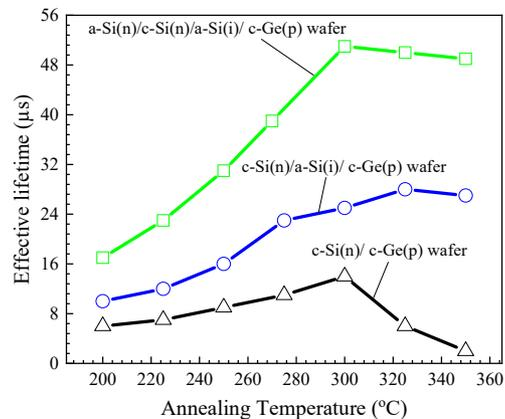
**Figure 4:** Effective lifetime measurements of three different configurations with c-Si(n) on c-Ge substrate as a function of the annealing temperature. For all samples, the rear side was coated by the dielectric stack a-SiC<sub>x</sub>:H(i)/Al<sub>2</sub>O<sub>3</sub>/a-SiC with a rear surface recombination velocities of 9 cm/s.
