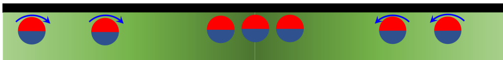
FIG. 6. 1D boundary layer chemotactic destabilization: a small disturbance in the particle distribution along the wall and the particles' activity introduce a local increase in solute concentration (green) and a small horizontal bias of the orientation of neighboring particles that start swimming toward and accumulating in this solute-rich region.
