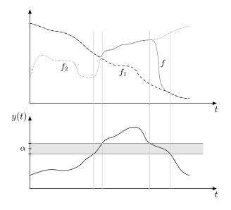
Fig. 6. Switching functions. Functions  $f_1$  and  $f_2$  are represented in the first graph by the dashed and dotted line, respectively. The resulting function is represented in gray. The second graph displays the control function y, where  $\alpha$  is the threshold.
