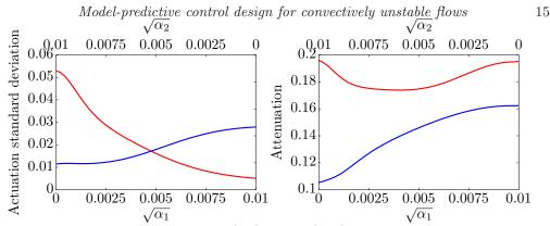
FIGURE 11. On the left: Actuations  $u_1$  (red) and  $u_2$  (blue) standard deviation when the flow is designed for actuation penalty weights  $\alpha_1 = 0.01 - \alpha_2$  varying from 0 to 0.01. On the right: Corresponding attenuation on  $y_1$  (red) and  $y_2$  (blue).
