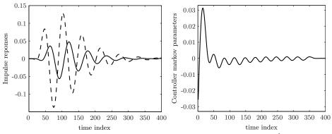
FIGURE 3. Left :Identified impulses responses,  $\mathsf{G}_{uy}$  (dashed) and  $\mathsf{G}_{wy}\mathsf{G}_{ws}^{-1}$  (plain). Right : computed impulse response of the controller  $\mathsf{C}_{su}$ .
