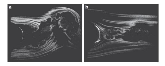
Figure 1.3: Flow past a cylinder at  $R_e = 33000$ . (a) uncontrolled, (b) controlled by plasma actuators aiming at separation control.
