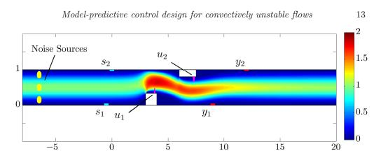
FIGURE 6. Flow in an obstructed two-dimensional channel; the base flow is visualized by the streamwise velocity, and the location of sensors and actuators is indicated.
