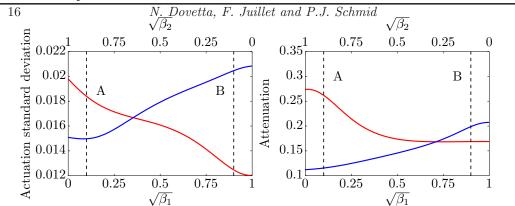
FIGURE 13. On the left: Actuations  $u_1$  (red) and  $u_2$  (blue) standard deviation when the flow is designed for objective sensor weights  $\beta_1 = 1 - \beta_2$  varying from 0 to 1. On the right: Corresponding attenuation of  $y_1$  (red) and  $y_2$  (blue).
