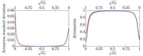
FIGURE 12. On the left: Actuations  $u_1$  (red) and  $u_2$  (blue) standard deviation when the flow is designed for actuation penalty weights  $\alpha_1 = 1 - \alpha_2$  varying from 0 to 1. On the right: Corresponding attenuation on  $y_1$  (red) and  $y_2$  (blue).
