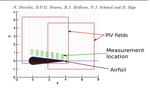
FIGURE 2. Experimental setup of the flow around an idealized airfoil, showing the spatial coverage of the flow by the cameras. The measurements taken from the flow and used in the data-assimilation are indicated by green square symbols.
