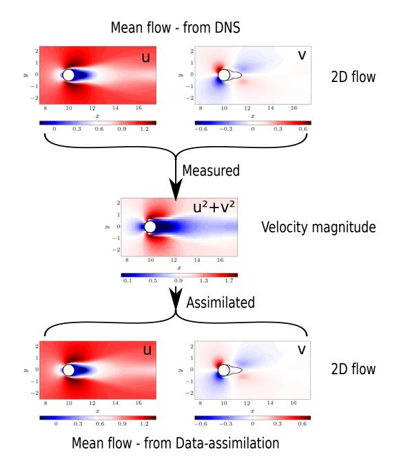
Figure 4.2: Mean velocity reconstruction by data-assimilation of velocity magnitude measurements. Top: initial mean flow from a direct numerical simulation, (left) streamwise velocity component, (right) normal velocity component; Middle: velocity magnitude on a coarsened grid, taken as the input to the assimilation algorithm; Bottom: reconstructed flow fields, (left) streamwise velocity component, (right) normal velocity component.
