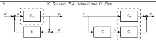
FIGURE 2. Feed-back (left) and feed-forward (right) control layout.  $G_i$  are transfer functions inherent to the system, K and C are the transfer functions of the respective controllers. The respective physical systems are enclosed by dashed lines.
