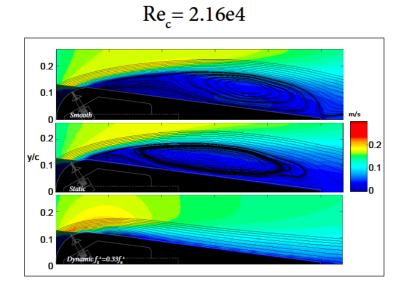
FIG. 2 – From [8], predetermined separation control. The colormap visualizes the mean velocity; stream lines are also plotted to highlight the recirculation bubble. The top plot shows the flow around a smooth airfoil; the middle plot shows the flow around the airfoil with static actuation; the bottom plot shows the flow around the airfoil with predetermined periodic actuation. In the latter case, the predetermined control successfully reattaches the flow.
