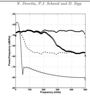
FIGURE 8. Power spectral density of the different measurement disturbances: crosses denote the white noise, circles show the colored noise 1, the dashed-line displays the colored noise 2. The spectrum of the noise-free output signal is represented by the solid line.
