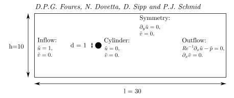
FIGURE 1. Sketch of the geometry of two-dimensional flow around an infinite cylinder. The full computational domain, the characteristic lengths and the applied boundary conditions are shown. The cylinder's diameter, the height and length of the domain d, h and l are given in nondimensional units.
