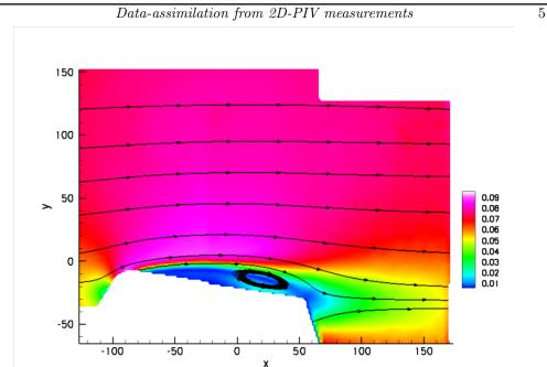
4.4. Article : Data-assimilation of a 2D PIV measurement over an idealized airfoil
