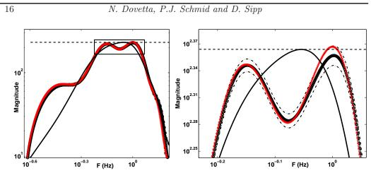
FIGURE 7. Bode diagram of the uncontrolled system (black line), the nominal CSTF (black thick line), and the exact CSTF (red); the error bounds around the nominal CSTF are shown by black mix-dashed lines. The maximum amplitude of the uncontrolled system is represented by a dashed horizontal line. (b) Magnified view of (a) for a limited frequency range.
