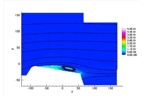
FIGURE 9. Color contours of the relative measurement error in percentage of the local velocity magnitude for flow around an idealized airfoil. Streamlines are shown in black.
