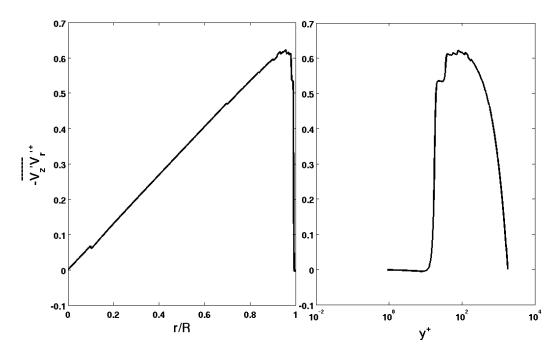
FIG. 3: Shear stress (normalized with the velocity scale  $u_{\tau}$ ) as a function of : the normalized radius (outer scale, left plot); the distance from the wall (inner scale, right plot).
