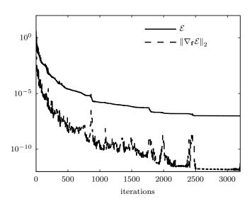
FIGURE 3. Convergence curves for full-identification case  $(\mathcal{M} = \mathcal{I})$ . The solid line represents  $\mathcal{E}$ , and the dashed line represents  $\|\nabla_{\mathbf{f}} \mathcal{E}\|_2$ .
