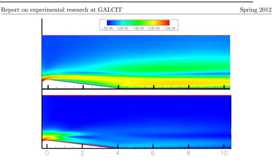
FIG. 10 – Uncontrolled (top) and controlled (below) flow around the airfoil. The colormap shows the fluctuations' intensity about the base flow. Applying a disturbance-rejection controller reduces the fluctuation intensity.
