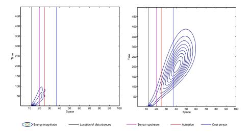
FIGURE 4. Controlled (left) and uncontrolled (right) impulse response (from the noise source) in a space-time diagram.
