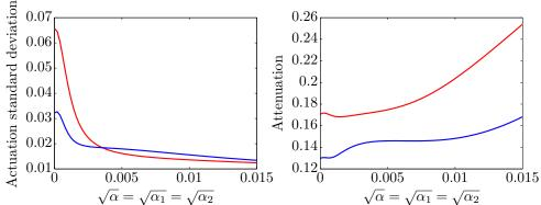
FIGURE 10. On the left: Actuations  $u_1$  (red) and  $u_2$  (blue) standard deviation when the flow is designed for actuation penalty weights  $\alpha_1 = \alpha_2 \equiv \alpha$  varying from 0 to 0.015. On the right: Corresponding attenuation on  $y_1$  (red) and  $y_2$  (blue).
