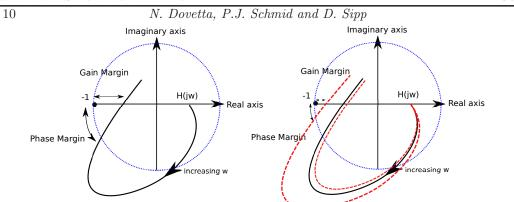
FIGURE 3. Nyquist plot of the *OLTF*, showing phase and gain margins, based on the nominal system (left) and the nominal system with uncertainty bounds (right).
