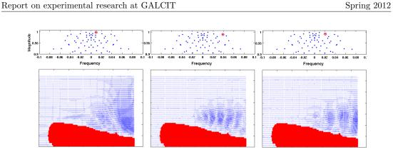
FIG. 7 – Eigenvalues and corresponding modes from a dynamic mode decomposition (DMD) of the TR-PIV data around the airfoil. The circled eigenvalue corresponds to the eigenmode plotted below.
