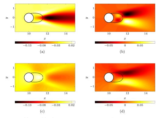
FIGURE 13. (a)  $\alpha$  and (b)  $\beta$  (respectively, left and right column) of the real reduced Reynolds stress tensor , and reconstructed tensor components (c)  $\alpha_{opt}$  and (d)  $\beta_{opt}$ . The dashed-lines indicate the extent of the recirculation bubble of the true mean-flow.
