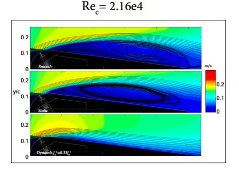
Figure 1.4: Separation control on an idealized airfoil using a predetermined control strategy, from Gonzalez *et al.* (2010). The colored contours represent the mean velocity; stream lines are also plotted to visualize the recirculation bubble. (top) uncontrolled flow around a smooth airfoil; (middle) flow around the airfoil with a static roughness element; (bottom) flow around the airfoil with a periodically activated roughness element. In the latter case the flow reattaches.
