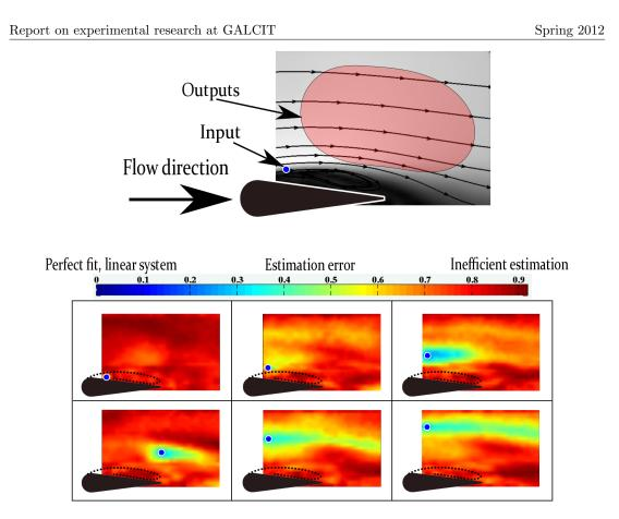
FIG. 11 - Linear identification error, the blue point is the chose input, the rest of the field represents the set of outputs.
