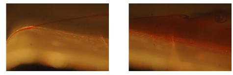
FIG. 8 – Dye streaks in the shear layer for flow around an airfoil with a splitter plate; the chord-based Reynolds number is  $Re_c = 10000$ .
