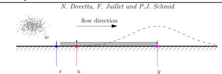
FIGURE 2. Setup of a control problem for the Ginzburg-Landau equation.
