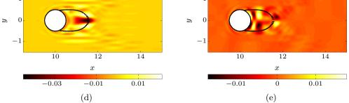
FIGURE 9. (a): Velocity magnitude measures on a mesh corresponding to n = 6. (b) and (c): Reconstructed field  $\mathbf{u}_{opt}$ . (d) and (e): Two components of the error  $\Delta \mathbf{u}$ . The dashed-lines in figures (b) and (c) represent the extent of the recirculation bubble for the reconstructed field. In figures (d) and (e), these lines have been reproduced along with those of the true recirculation bubble.
