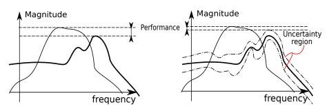
FIGURE 4. Bode diagram of the uncontrolled (thin black) and controlled (thick black) transfer function, showing  $H_{\infty}$ -based performance of nominal system (left) and the nominal system with uncertainty bounds (right).
