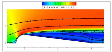
FIGURE 4. Base flow for  $Re_c = 12500$  from the solution of the RANS equations with  $\mathbf{f}_s = 0$ . The color contours display the velocity magnitude; streamlines are indicates as black lines. This flow field acts as the starting point of the iterative data-assimilation algorithm.
