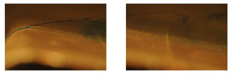
FIG. 9 – Dye streaks in the shear layer for flow around an airfoil with a splitter plate; the chord-based Reynolds number is  $Re_c = 25000$ .
