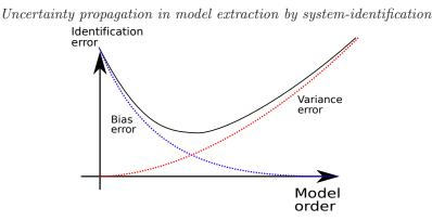
FIGURE 1. Sketch of the variance and bias error contribution to the total estimation error, as a function of the model order.
