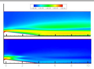
Figure 3.1: Numerical simulations of the linearized Navier-Stokes equations for flow around an idealized airfoil (chord Reynolds number  $Re_c = 2000$ , uncontrolled (top) and controlled (below) configurations. The colormap shows the local kinetic perturbation energy. Applying a disturbance rejection controller effectively reduces the fluctuation intensity.
