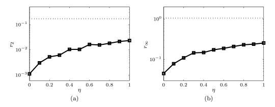
FIGURE 10. Results for the noise reduction case. The error (measured relative to the base flow error)  $\|\Delta \mathbf{u}\|$  is plotted (square symbols) against the noise strength  $\eta$  in the measured signal. The error made by approximating the mean flow by the base flow is represented with a dashed line. (a)  $r_2$  error, (b)  $r_{\infty}$  error as defined in (4.1).
