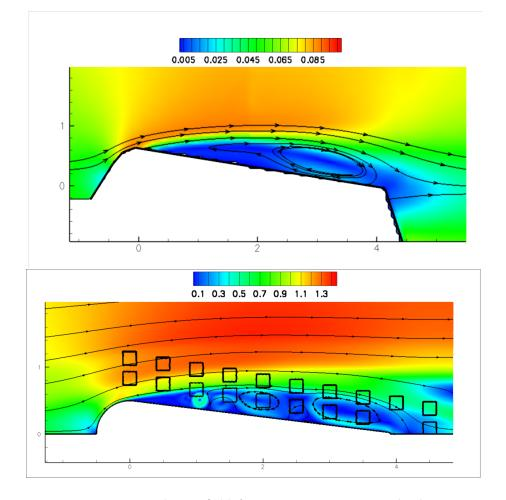
Figure 4.3: Top: mean velocity field from averaging time-resolved PIV measurements, visualized by color contours of the velocity magnitude and streamlines; Bottom: reconstructed flow field using data-assimilation, visualized as above. The black squares indicate the measurement locations that serve as input to the dataassimilation algorithm.
