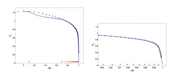
FIG. 1: Mean-velocity profile  $V_z$  versus the normalized radius r/R. Black symbols indicate true measurements, while the blue line displays the reconstructed mean-velocity profile using data-assimilation of a restricted set of measurements. The radii where velocity measurements entered the data-assimilation algorithm are shown as the red circles. (Left) mean-velocity profile over the entire pipe radius, (right) magnified region close to the pipe wall.
