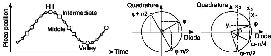
Fig. 2. On the left is a schematic of the piezo oscillation in time. Points on the curve indicate acquisition times. Hollow circles and squares show two groupings for calculating quadratures. The two plots on the right show data points in complex space. The real component is the scaled diode measurement. The imaginary component is the calculated quadrature.
