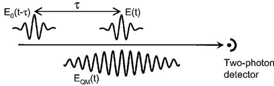
Fig. 2. Time-domain HOT SPIDER. The second-order nonlinear signal is recorded by a two-photon time-integrating detector as a function of time delay  $\tau$  between a reference pulse,  $E_0$ , and a superposition of two pulses: the pulse to be measured,  $E$ , and a quasi-monochromatic pulse,  $E_{QM}$ .
