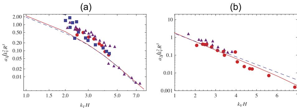
FIG. 8. Measurement of  $a_1$  (a) and  $a_2$  (b) vs depth. The symbols represent the sphere diameters, “•” 1 cm, “■” 2 cm, and “▲” 3.76 cm. The lines are the prediction of the mirror-dipole approximation. Solid line: numerical calculation of the integral [Equation (5)]. Dashed line: long range expansion, Equations (15) and (16). We keep here only the experimental points for which  $H$  is larger than  $2R$ .
