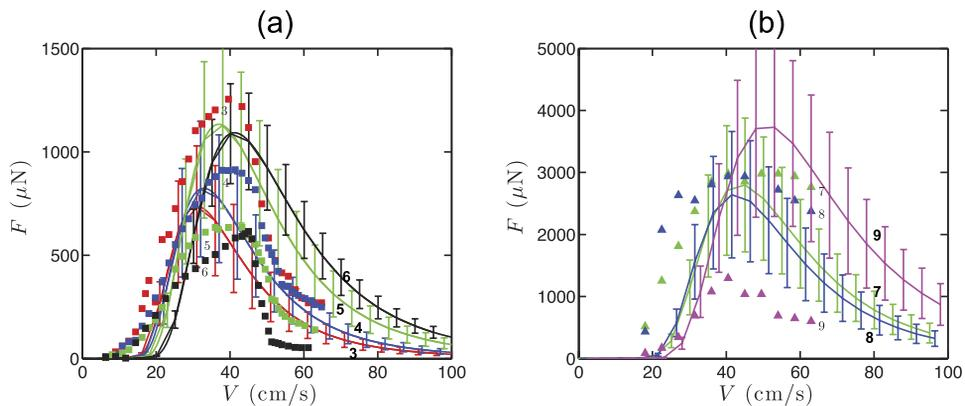
FIG. 11. Comparison of the measured wave drag (symbols) and the theoretical prediction (lines) as a function of the velocity for 2 cm spheres (a) and 3.76 cm spheres (b). The depths of measurement (numbering in regular for measurements and bold for prediction) are indicated in Table I. The theoretical curves are rescaled by a factor  $(a^*/a_1)^2$ , estimated at 29.24 cm/s (a) and 45 cm/s (b), and error bars are based on the error in this rescaling.
