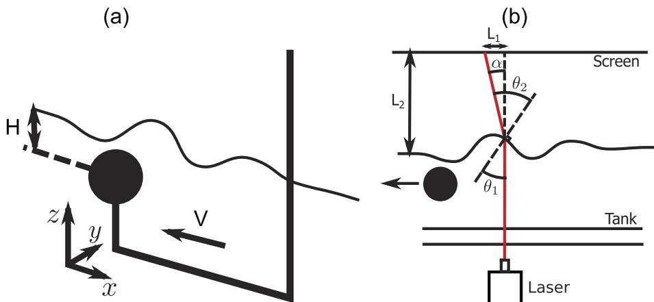
FIG. 5. Schematic of the wake measurement apparatus: (a) general view and (b) side view and conventions.
