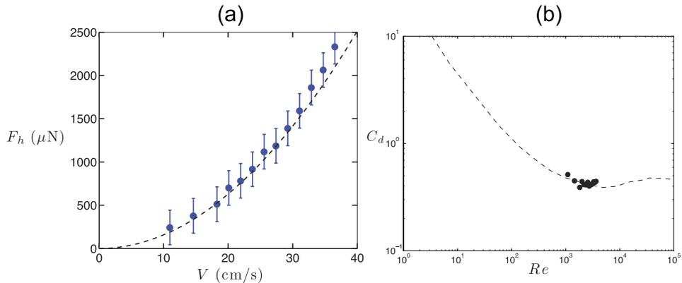
FIG. 2. (a) Hydrodynamical drag of a 2 cm diameter sphere. The dashed line is an estimation through the equation  $F_h = \frac{1}{2}\rho V^2 \pi R^2 C_d$ , with  $C_d = 0.5$ . The error bars represent the sensibility of the apparatus. (b)  $C_d$  as a function of  $Re$ ; dots: measurements, dashed line: data from the literature.<sup>17</sup>
