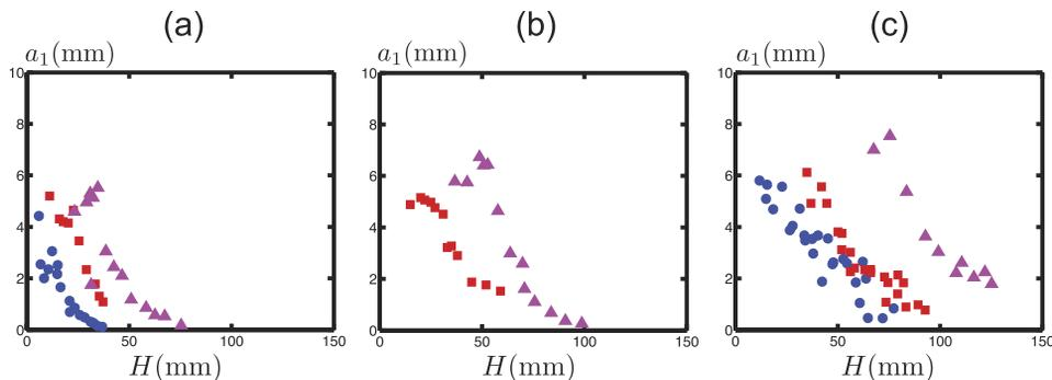
FIG. 7. Amplitude of the wake  $a_1$  as a function of the depth, for three sizes of sphere. The symbols represent the sphere diameters, “•” 1 cm, “■” 2 cm, and “▲” 3.76 cm. The velocities are (a)  $V = 29.2$  cm/s, (b)  $V = 45$  cm/s, and (c)  $V = 60$  cm/s.
